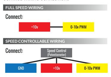
**NOTE:** 0-10 volt analogue signal supplied by fan motor. 3 wire low voltage cable or Cat 5 or Cat 6 cable to be used to either an Airius Potentiometer or a BMS controller (by others).
